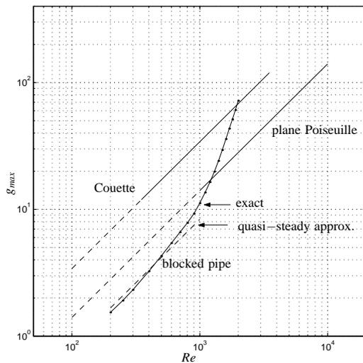
Figure 4: Maximum transient growth  $g_{\max} \equiv \max\{g^*\}$ . Corresponding results from Couette and plane-Poiseuille flows are provided for comparison (solid and dashed sections correspond to transitional and unstable flow, respectively).
