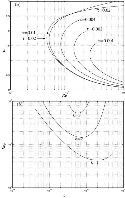
Figure 2: Plots of (a) Neutral-stability curves for blocked-pipe flow and (b) the corresponding critical Reynolds number for azimuthal wavenumbers  $k = 1, 2, 3$ . The solid line corresponds to the neutral-stability curves.
