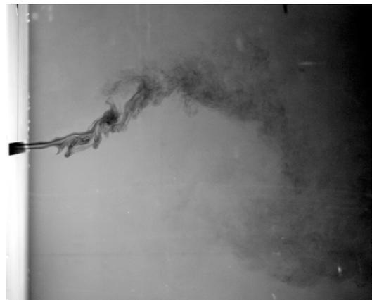
Figure 4. Jet in the weaving jet regime with inclusion of the flow field further downstream. Initially nearly straight jet shows high degree of oscillation in the far field.
