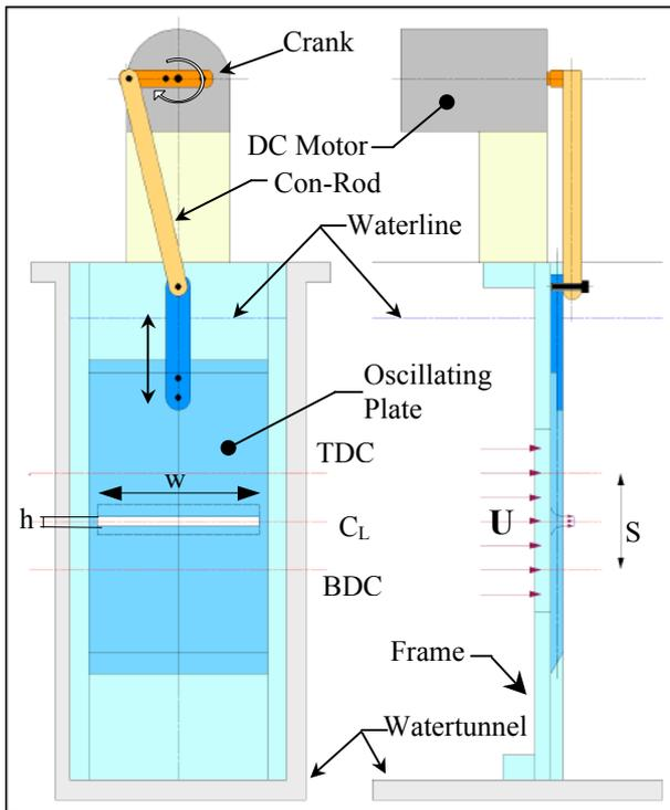
Figure 1. Mechanically Oscillating Planar Jet mechanism.  $S$  = oscillation stroke;  $C_L$  = oscillation centreline; TDC = top dead centre; BDC = bottom dead centre;  $h$  = nozzle width;  $w$  = nozzle length;  $U$  = jet mean velocity.
