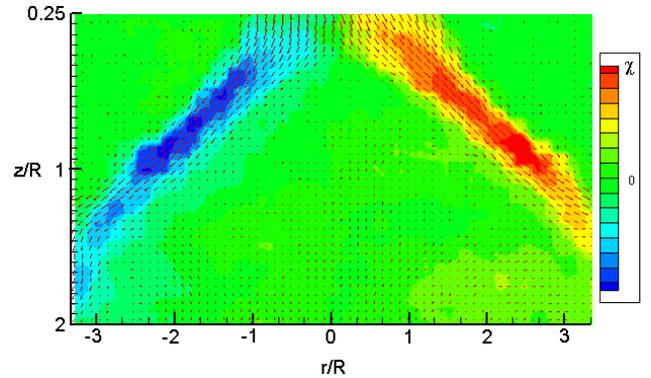
Figure 4: Vorticity  $\chi$  plot of a swirling jet undergoing breakdown with no pulsing ( $m_v=0$ ) at  $Re=600$   $S=1.36$ .
