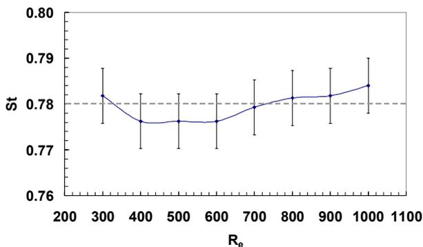
Figure 3: Shear-layer Strouhal number as a function of Reynolds number.  $St_n$  is shown by a dashed line.
