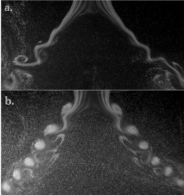
Figure 6: (a) Unpulsed breakdown  $m_0=0$  at  $Re=600$ ,  $S=1.41$ ; (b) pulsed breakdown  $m_0=6\%$ ,  $St=0.78$  at  $Re=600$ ,  $S=1.41$  clearly showing increased vorticity concentrations in the shear layer resulting in increased  $\Delta Z_{bp}$ .
