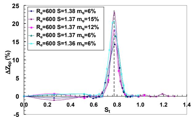
Figure 5: Pulsed breakdown position  $Z_{bp}$  as a percentage of the un-pulsed breakdown position  $Z_b$  (where:  $\Delta Z_{bp} = (Z_{bp} - Z_b) / Z_b$ ) for various Swirl and PMFV values at  $Re=600$ . Similar results occur for the other Reynolds numbers tested.
