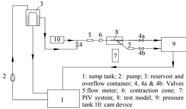
Figure 2: Schematic presentation of in-vitro experimental arrangement.
