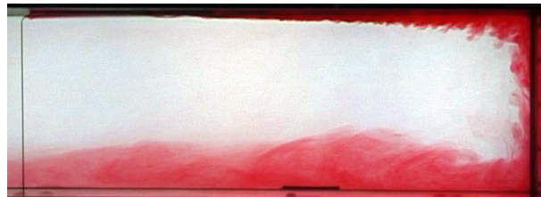
Figure 1: Dye visualisation of the convective flow driven in a box by differential heating along the lid [5]. In this experiment surface heat fluxes q_h and q_c (= -q_h) per unit box width are applied over the left- and right-hand halves of the lid, respectively. The field of view shows only the right-hand (cooled) end of the box. The thin vertical line at the left of the photograph corresponds to the centre of box, where dye was introduced into the boundary layer adjacent to the lid. Heat is transferred to/from this boundary layer, maintaining a horizontal density gradient and a flow directed from the heated region to the cooled region (left to right). A turbulent outflow from the plume is visible at the base of the box, directed from right to left. For sufficiently large heat fluxes most of the temperature variation occurs across the lid boundary layer, which occupies a small fraction of the total depth.
