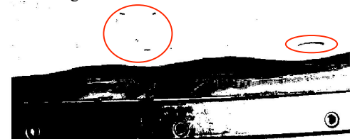
Figure 5: Black and white reduction of the green channel data, note the metallic base of the flume with bolts along the bottom of the image. The ellipsoid indicators show where marks on the flume need to be masked. The flow is moving from left to right in this image
