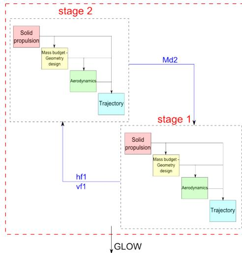
Figure 3: Design Structure Matrix of the sounding rocket
