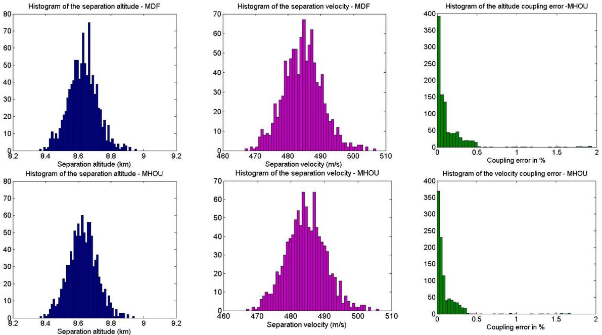
Figure 7: Altitude (blue) and velocity (pink) couplings in MDF and MHOU formulations + coupling error (green)
