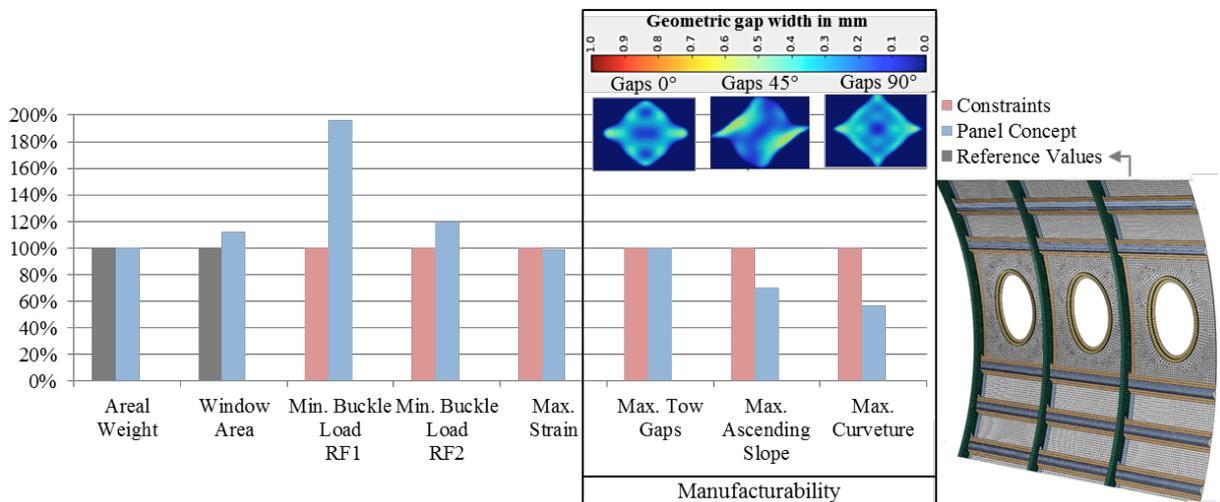
Figure 6: Optimisation result with constraints and reference panel (right) and true geometric gap fields on peaks
