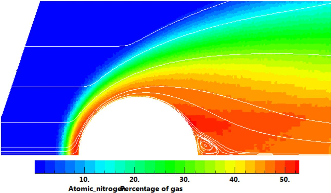
The second set of contours employs the “continuum data” option. The vibrational collision rate was again based on Equation (1), but with  $T$  given by the overall flow temperature. The total collision energy model was applied to the following rate coefficients in SI units.
