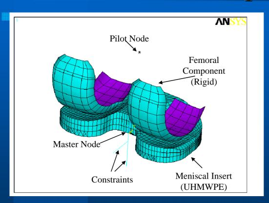
ANSYS software was used for all finite element modelling
