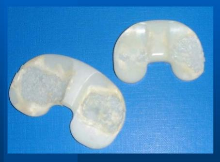
Most common failure in a TKR is due to the deterioration of the UHMWPE meniscal insert. This is due to geometric deformation, adhesive wear, surface pitting, 3 body abrasive wear, and most destructive -DELAMINATION
