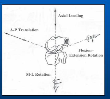
•Medial-Lateral Rotation –the motion as the knee internally or externally rotates, again this motion is restricted by ligaments and geometry of the end of the tibial bone
