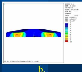
a. Contact Stress on size 3 6mm meniscal insert (M3) when loaded at 3\*Body Weight with a size 3 femoral component (F3)
