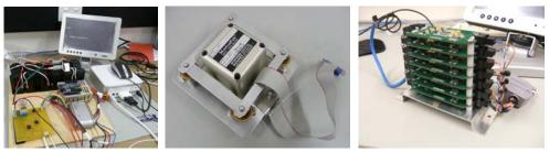
The Jabiru Flight Laboratory is based on the School's J400 four seat Jabiru. This has being fitted out with a glass cockpit avionics system, a suite of flight sensors and a data acquisition system to measure all flight characteristics. The complete system will provide a flight test capability that will facilitate teaching and learning in flight test techniques, as well as research into flight stability, avionics systems and flight control system development.
