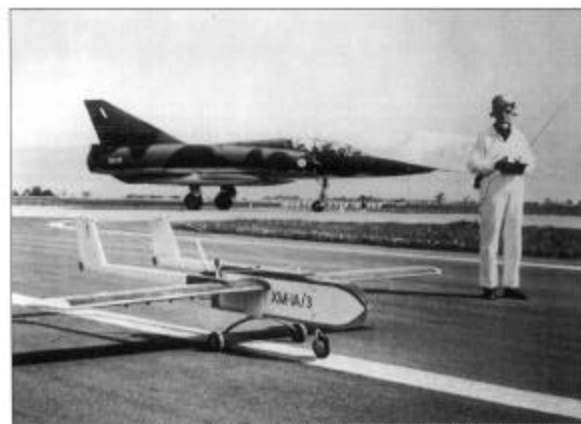
Brian Hancock with R.P.V. XM-1A/3. This machine was fitted with a 50hp, 49cc, Kadabo engine using a 20" dia. x 1 1/2" propeller. A.E.W. 41 hp. This version also has the high speed "self flying" mechanism. Photo taken on R.A.A.F. Base, Edinburgh with A.M.D.C.'s 2nd unit Manager looking on.
