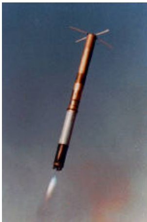
Figure 4 Nulka hovering rocket decoy
