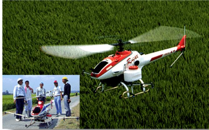
**Figure 2** Yamaha industrial-use unmanned helicopters at work
