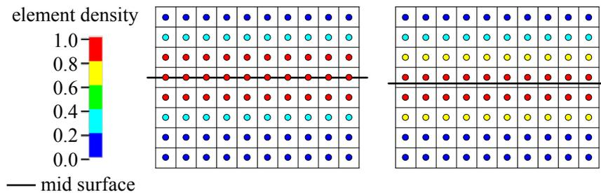
Figure 3: Movement of mid surface through change of elements densities
