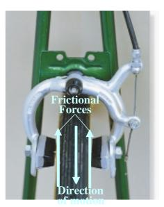
Impending motion: Impending motion refers to the state just before surfaces start to slip. In this case the static frictional force has reached its upper limit and is given by the equation:
