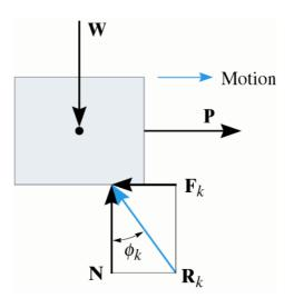
Tipping: When an object starts to tip, it starts to pivot around a point. As a result the contact forces (frictional and normal) must be applied at the pivot point. If the object tips before it slips, then one can find the frictional force from the equations of equilibrium.
