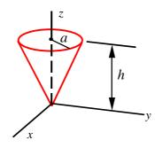
Calculate the mass moment of inertia of the cone about the *z*-axis. Assume the cone is made of a uniform material of density  $\rho$  (mass per unit volume).
