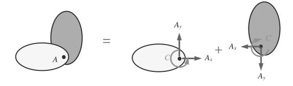
Forces and couples on a free-body diagram (FBD): Each force or couple on a FBD represents a model of how the body in the free-body diagram is effected by its surroundings. In selecting the forces and couples that are to be applied follow these steps:
