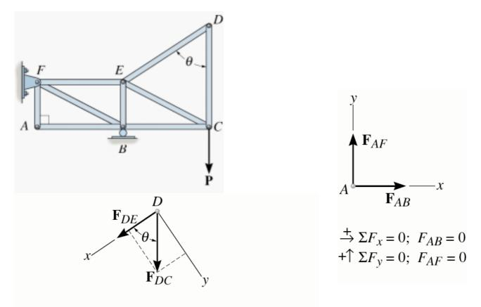
$\begin{aligned} +&\searrow \Sigma F_y = 0; \ F_{DC} \sin \theta = 0; \ F_{DC} = 0 \text{ since } \sin \theta \neq 0 \\ +&\swarrow \Sigma F_x = 0; \ F_{DE} + 0 = 0; \ F_{DE} = 0 \end{aligned}$
