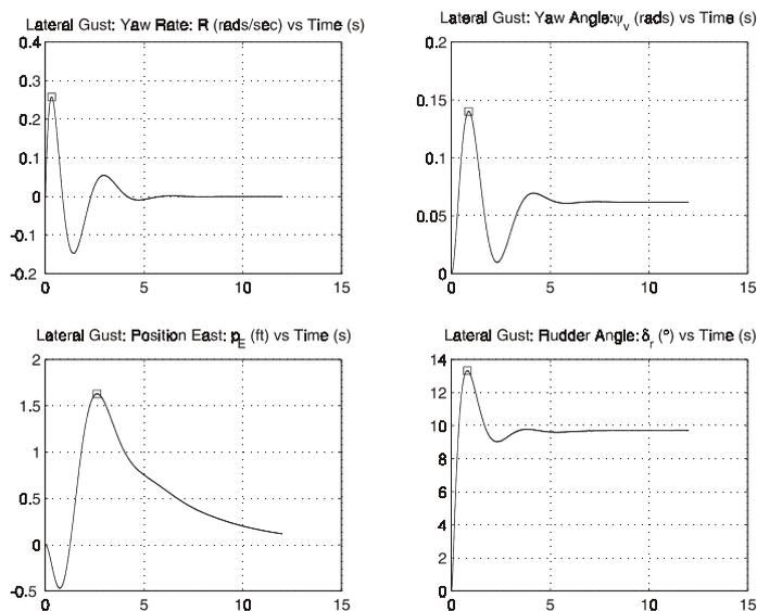
**Figure 9: Typical Lateral Step Response: 10 knot Side (East) Wind Gust.**
