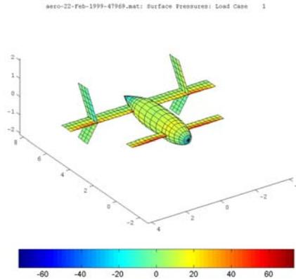
**Figure 8: Aerodynamic Model of Vehicle, (Dimensions in ft; Pressure in psf)**
