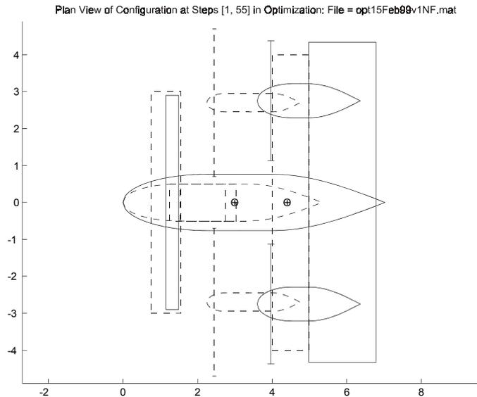
**Figure 10: Before and After Vehicle Profiles for a 50-lb Payload 600-Mile Range Vehicle, (dimensions in ft).**
