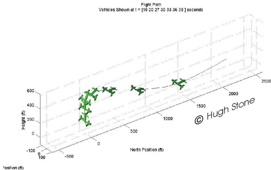
**Figure 11: Typical Simulation of Vertical to Horizontal Transition Under Automatic Control: (unequal time increments).**
