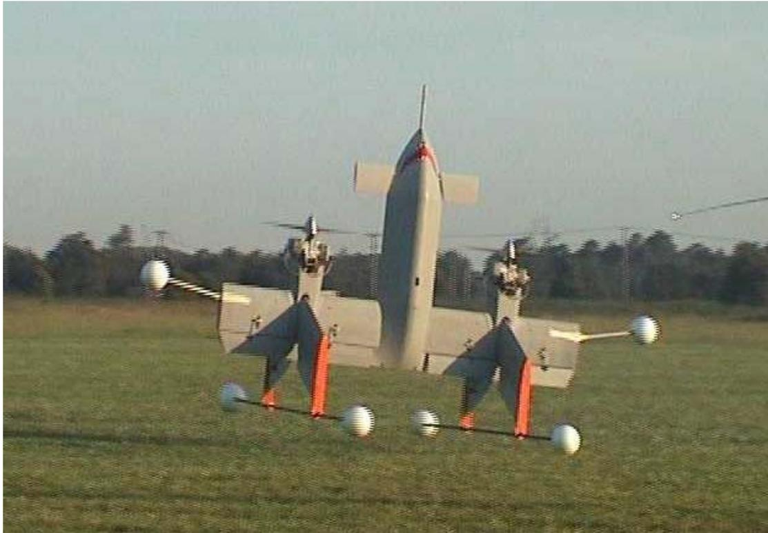
**Figure 7: First Free Flight of T-Wing Technology Demonstrator Vehicle under Manual Control. (Note "training" undercarriage").**
