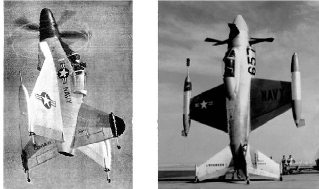
**Figure 2: Convair XF-Y1 and Lockheed XF-V1 Tail-Sitter Aircraft.<sup>1 2</sup>**
