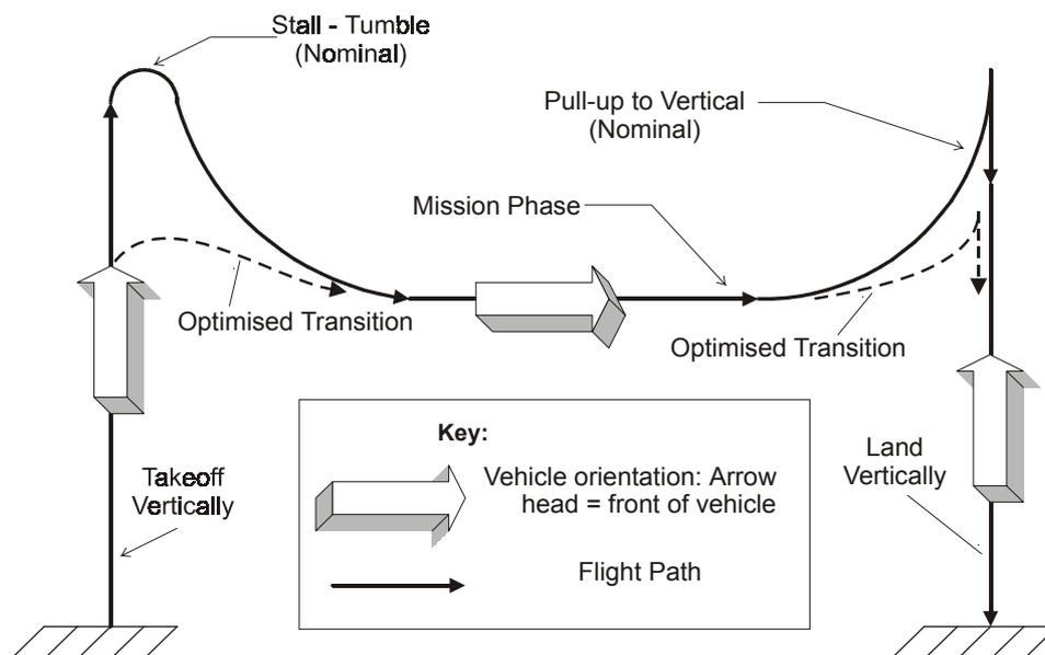
**Figure 5: T-Wing Vehicle Flight Path**
