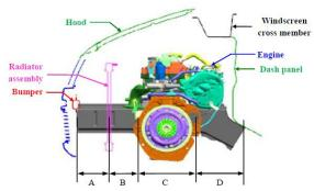
Figure 6: Crush spaces for front end structure
