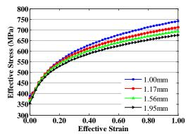
Figure 8: Effective stress-effective strain curves of HSLA340
