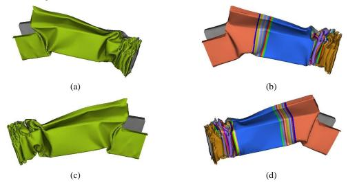
Figure 15 Comparison of the numerical result before and after optimization: (a) Left FLB of baseline design; (b) Left FLB of optimal design; (c) Right FLB of baseline design; and (d) Right FLB of optimal design
