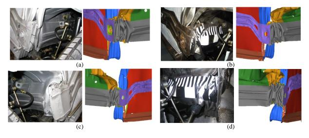
Figure 4: Comparison of FLB deformation patterns: (a) Left FLB of full-scale vehicle; (b) Left FLB of simplified frontal impact model; (c) Right FLB of full-scale vehicle; and (d) Right FLB of simplified frontal impact model
