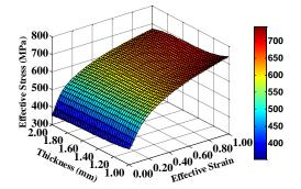
Figure 9: Effective stress-strain field of TRBs made of HSLA340
