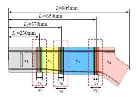
Figure 12: Geometry parameters of TRB FLB-inner
