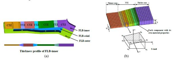
Figure 10: (a) Geometry model of TRB FLB-inner; and (b) FE model of TRB
