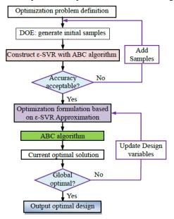
Figure 11: Flowchart of optimization process
