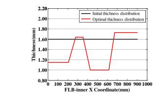
Figure 14: Thickness profile of TRB FLB-inner
