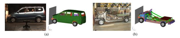
Figure 2: Physical model and FE model under 100% frontal impact: (a) full-scale vehicle; (b) simplified frontal impact model
