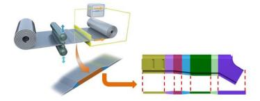
Figure 7: The schematic diagram of manufacturing process for FLB-TRB.
