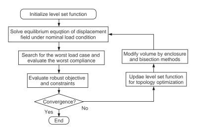
Figure 4: Flowchart of robust topology optimization
