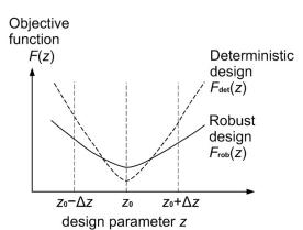
Figure 1: Concept of robust optimization
