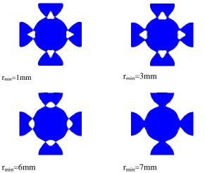
Figure 3: The effects of filtering radius on the optimal topology
