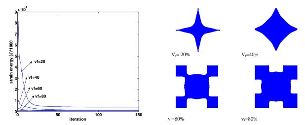
Figure 4: Variations of strain energy versus iteration for different  $V_{\rm f}$  Figure 5: Different optimal shapes with different  $v_{\rm f}$
